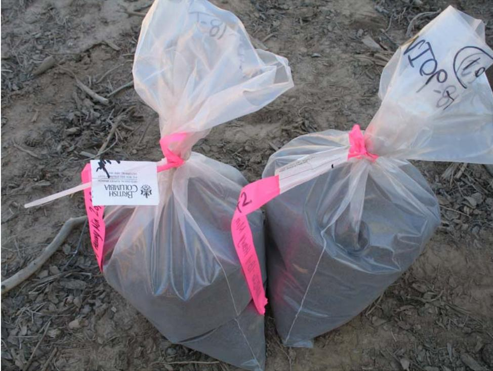
***Photo 5. Approximately 2kg of dry sieved sample from the bottom of each of the five pits are combined, stirred and poured into tamper-proofed bags. These are reinforced by placing them into a second bag. The two doubly-bagged parts of the sample are placed into clean plastic buckets, which are capped and taped for shipping.***
