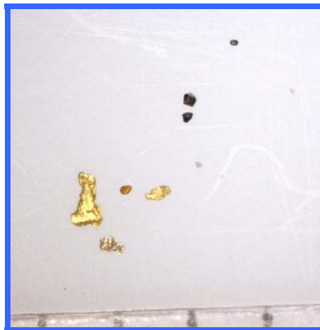
Figure 4: Gold grains in the heavy mineral concentrate of a bulk sediment sample at site 93G071006.
