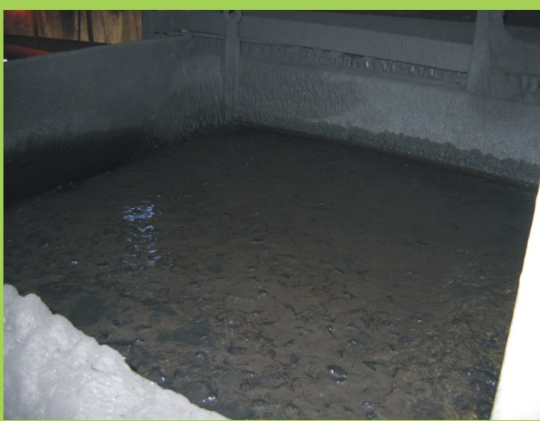
Fig. 4b Magnetite is used as a heavy media to separate coal from waste.
