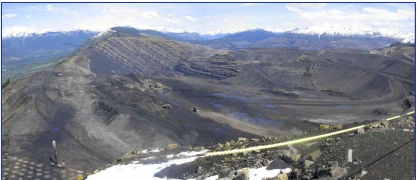
*Figure 83. (Below) The Greenhills coal mine has carved large open pits into a high ridge of coal-bearing sandstone and shale. The coal mines occur on ridges of sandstone and shale where the coal is near surface and can be mined by large open pits. The mine is surrounded by the high limestone peaks of the Rockies.*
