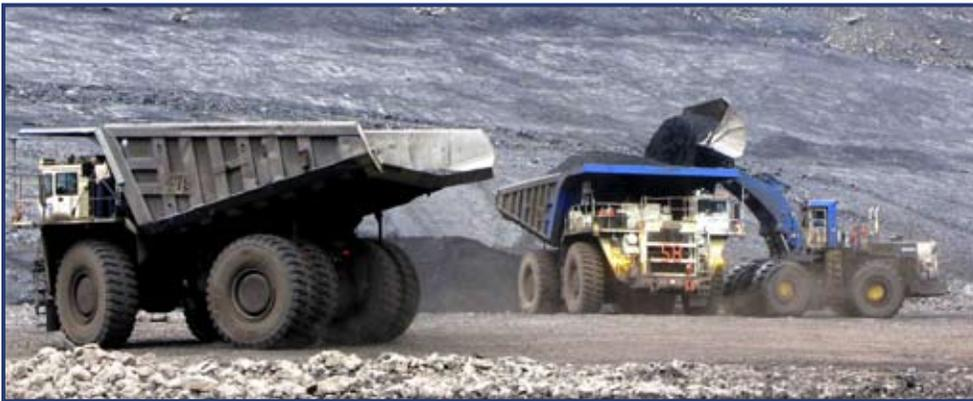
*Figure 82. Giant trucks carry coal from the bottom of the open pit mine to the mill.*
