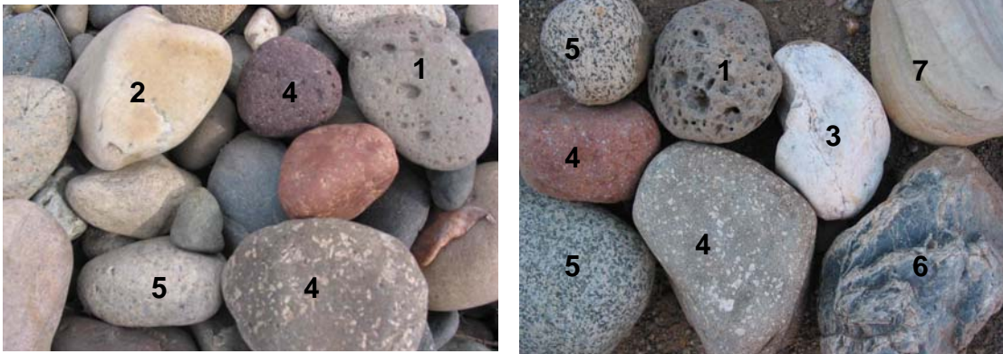
Figure 11. Different types of pebbles in gravel. 1, volcanic lava with gas bubbles. 2, quartzite. 3, quartz. 4, volcanic lava. 5, granitic rock. 6, chert. 7, mudstone.
