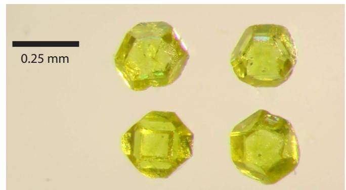
**Fig. 13.** Synthetic diamonds recovered from sample 17TFE0002. These are contamination from diamond drill bit and were recovered from each of 14 samples collected.
