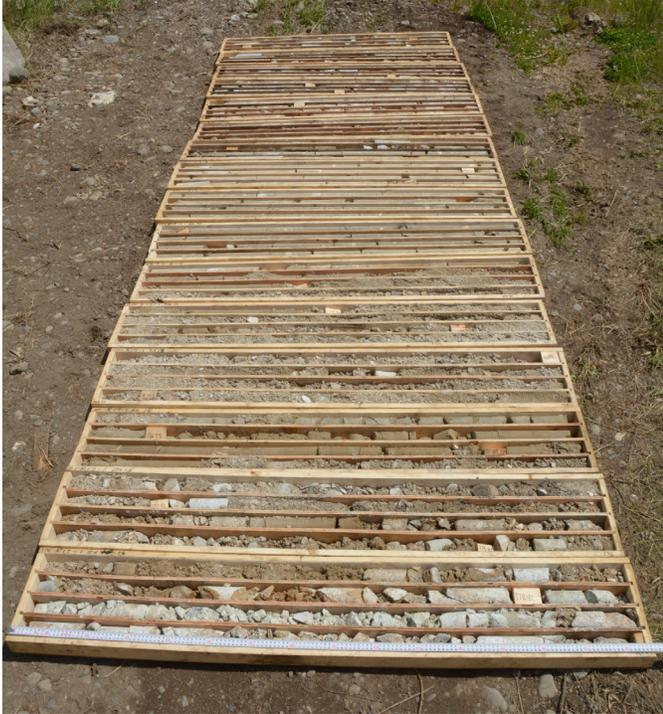
**Fig. 2.** Core boxes 1 through 17, from 0 m (top of photo) to 174 m (bottom of photo), for Happy Creek Minerals Ltd. diamond drill hole R17-01 (NQ size).
