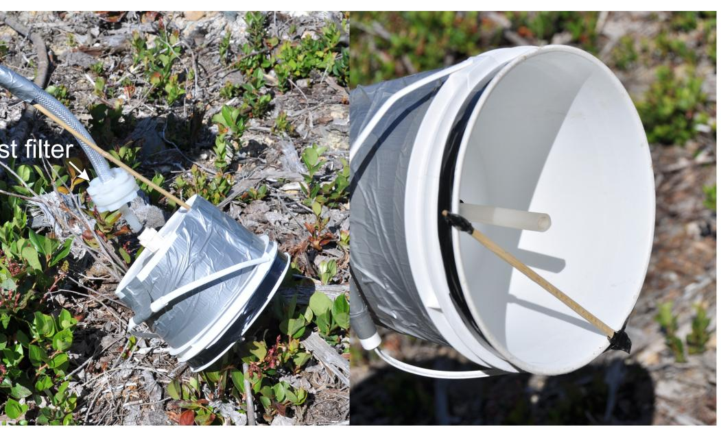
We sampled air 1 cm above ground under a bucket to minimize wind influence on GEM concentration. We used the average of 60 or 120 readings (1 second each) per station every 5 to 25 m along foot traverses.
