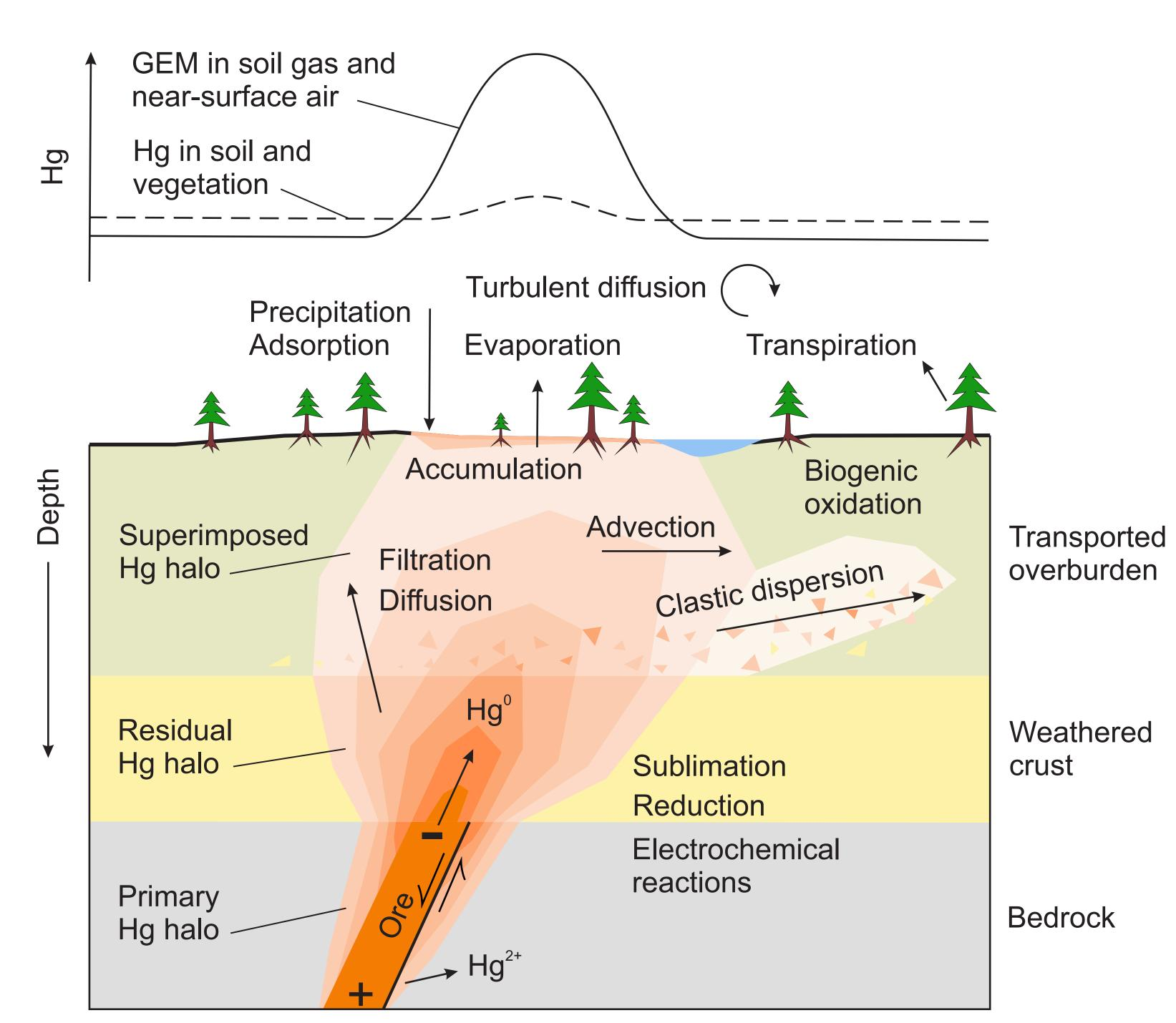
Model illustrating Hg dispersal from a drift-covered ore deposit and the processes forming Hg haloes in the surface environment. Schematic cross-section showing primary Hg halo of a partly eroded ore, residual Hg halo in weathered crust, and superimposed Hg halo in a transported overburden. The GEM halo in air is directly above the ore, because wind and turbulent air movement remove and dilute GEM.
