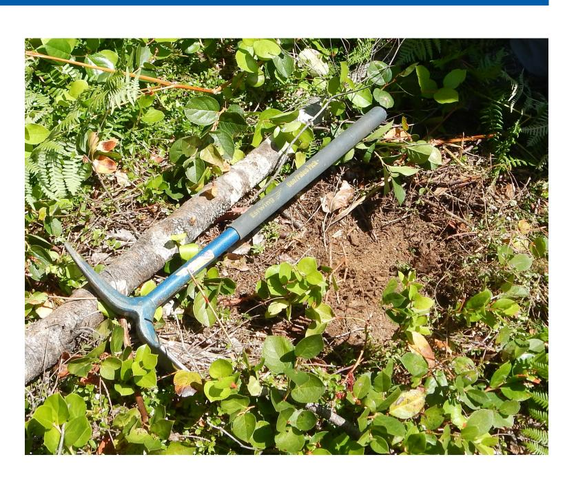
Before sampling GEM above overburden, we disturbed surface sediment mechanically with a hoe pick to release Hg<sup>0</sup> adsorbed in soils and vegetation.
