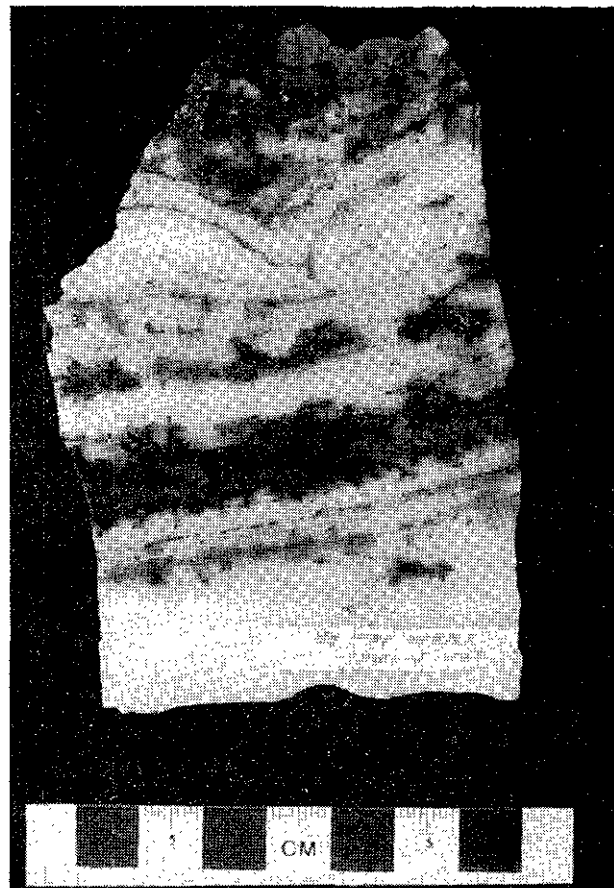
Plate B-6-12. Banded quartz-pyrite-galena-sphalerite-chalcopyrite veins from dump at the Joshua shaft (93), Stump Lake.
