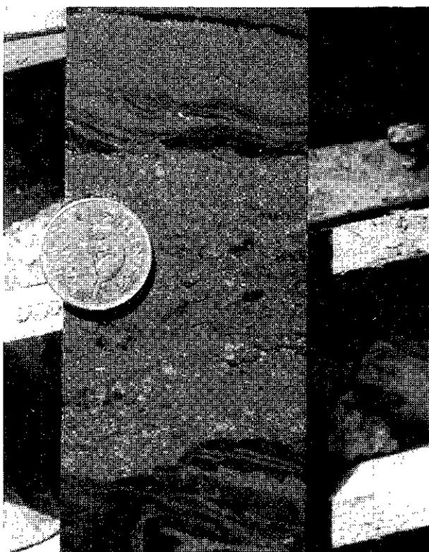
Plate B-14-5. Mudstone fragments in massive sulphide layer of the contact unit, southern 21B deposit, Eskay Creek (DDH CA89-87: 97 m).
