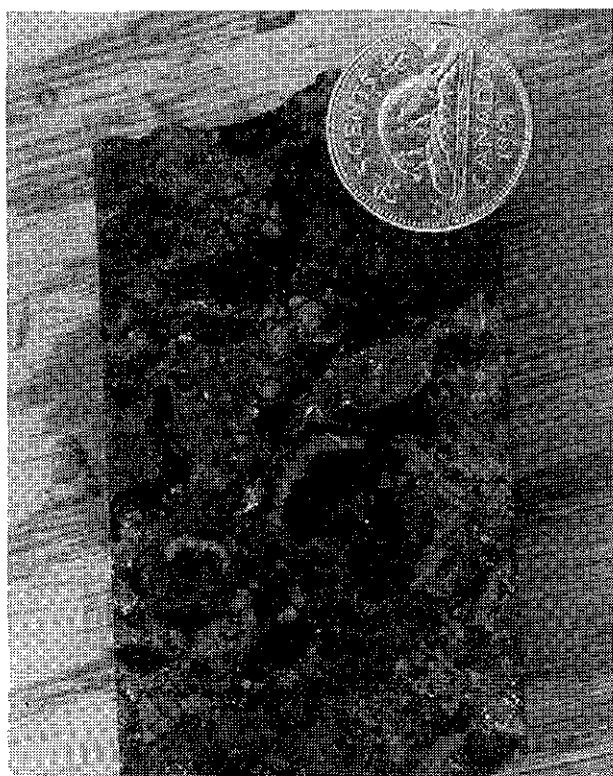
Plate B-14-6. Sulphide-rich vein with coarse-grained galena and zoned sphalerite, northern 21B deposit, Eskay Creek (DDH CA89-109: 90.5 m).
