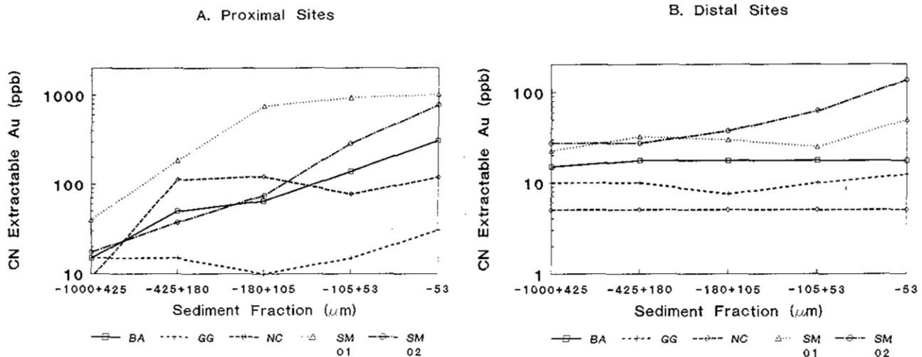
Figure B-5-3. Cyanide-extractable gold concentrations in placer tailings sediment fractions. BA = Ballarat mine, GG = Gallery Gold mine, NC = Nelson Creek mine, SM = McKeown mine (Spanish Mountain).
