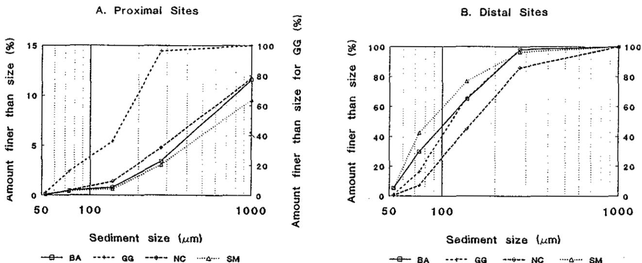
Figure B-5-2. Cumulative size distributions for proximal and distal placer tailings. BA = Ballarat mine, GG = Gallery Gold mine, NC = Nelson Creek mine, SM = McKeown Mine (Spanish Mountain).
