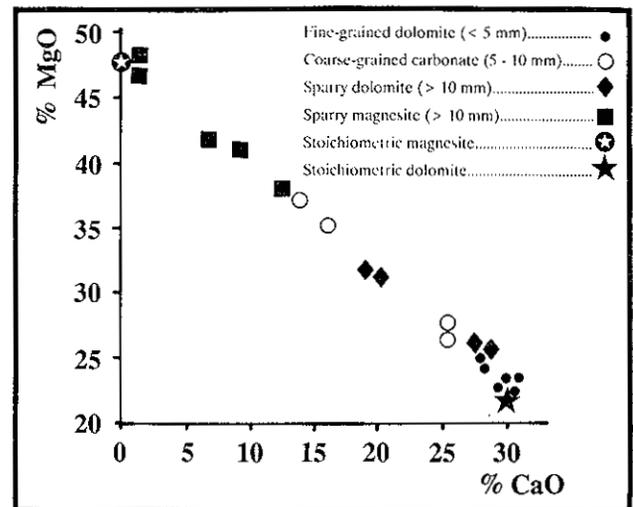
Figure B-1-2. Relationship between MgO and CaO content of carbonate rocks, Mount Brussilof area. The distribution of the data confirms that representative samples were collected (after Simandl and Hancock, 1991).
