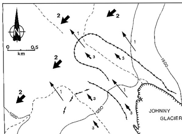
Figure B-7-10. Generalized glacial-flow history for the Johnny Mountain area. Long, thin arrows (1) illustrate early stage of cirque-glacier flow, thick arrows (2) indicate late stage of ice-sheet flow; both episodes presumed to have occurred during the Late Wisconsinan. Intermediate size arrows (3) indicate Neoglacial ice-flow of Johnny Glacier.
