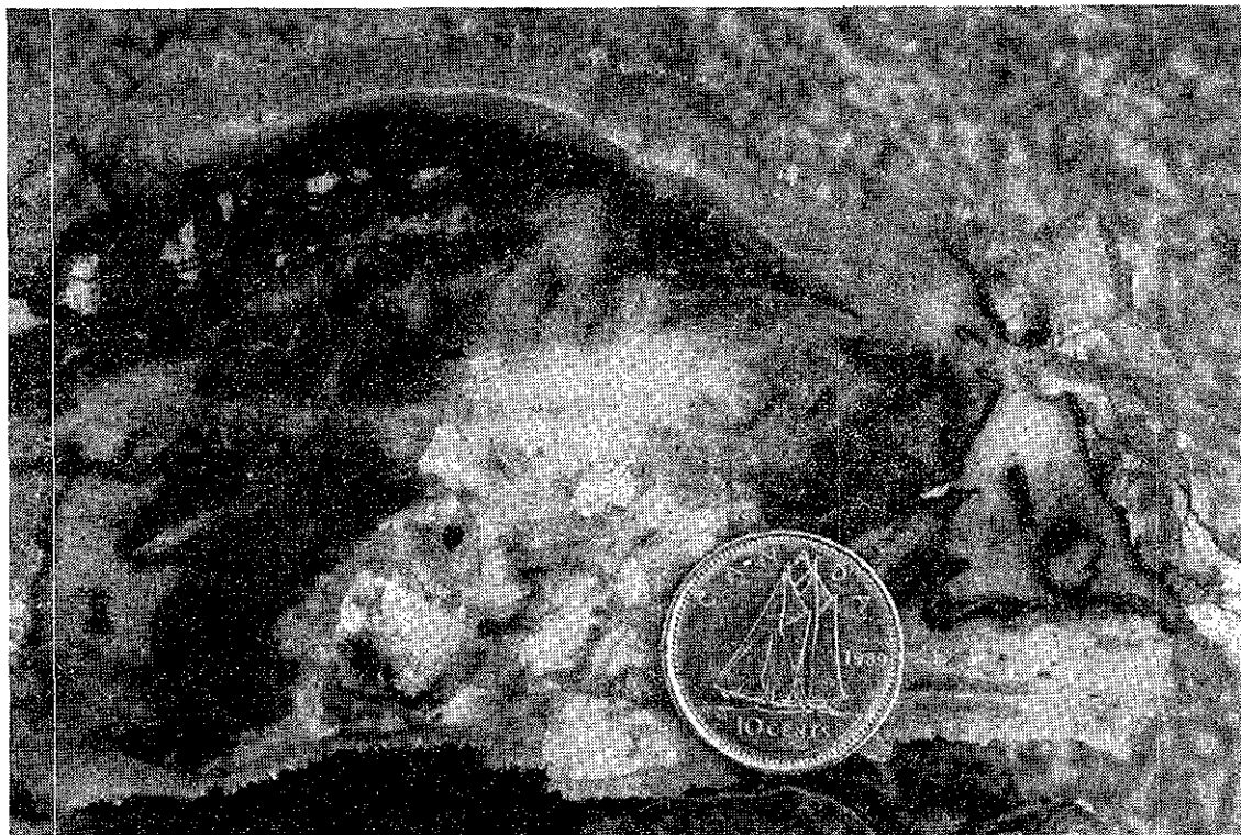
Plate B-9-9. Cut sample from the South zone displaying pervasive silica replacement of rhyolitic protolith by dark chalcedonic and clear drusy quartz phases. Note quartz pseudomorphs after coarse-bladed calcite, well-developed comb quartz on margins of sample and crustiform texture. Extremely fine grained pyrite occurs with chalcedonic quartz.
