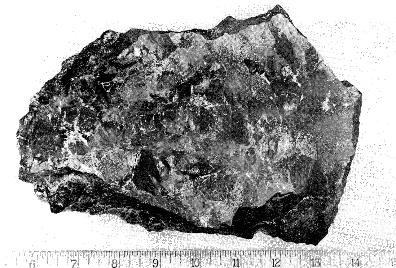
Plate 3. Red Mountain breccia on the northeast margin of the Marc zone. Angular grey to black siltstone fragments with heavily disseminated pyrite, pyrrhotite and sphalerite. Textures not apparent in the photograph indicate sphalerite and pyrrhotite are later than pyrite.
