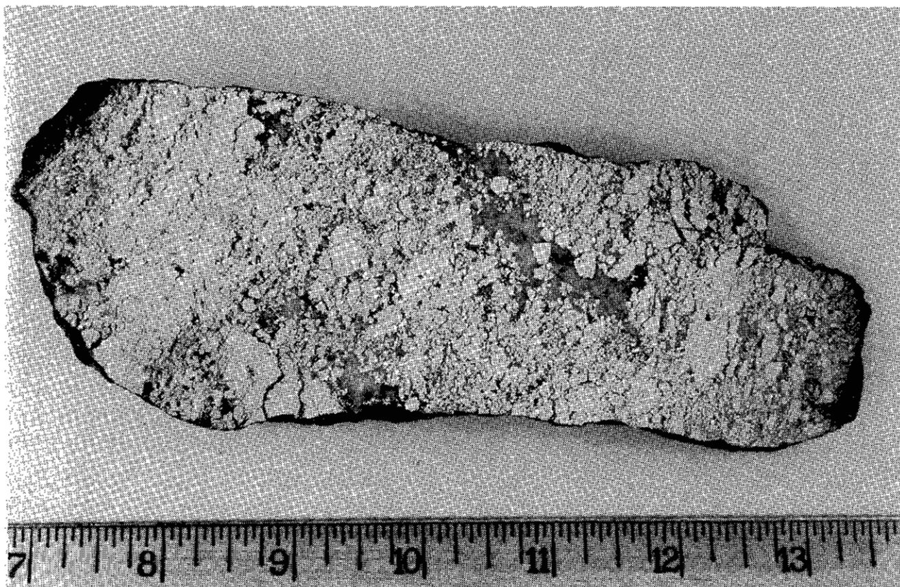
Plate 2. Red Mountain, Marc zone, 1100 crosscut. Coarse, massive pyrite with quartz gangue and showing fractured texture.
