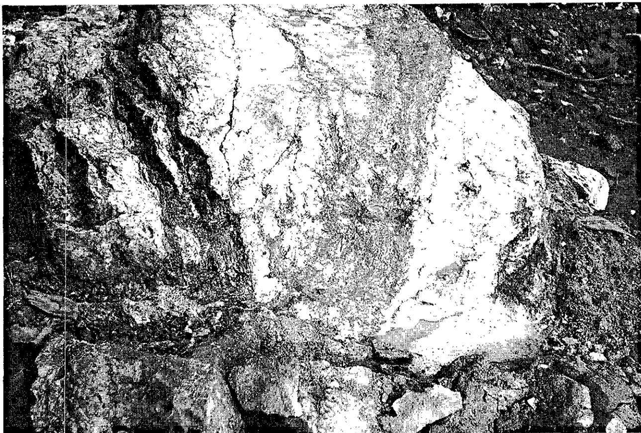
Photo 3. An example of sulphide-rich vein material from the 3B vein. The grey zone in the centre of the quartz-sulphide vein is fine-grained galena. This vein is in contact with the 155 fault (distorted argillite on left side of photo). Width of photo is about 1 metre.
