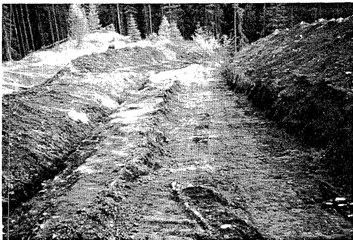
Figure 7. Small pit on the main coal seam, Tulameen Coal property. Coal layers (black) are separated by shale and bentonite (grey).
