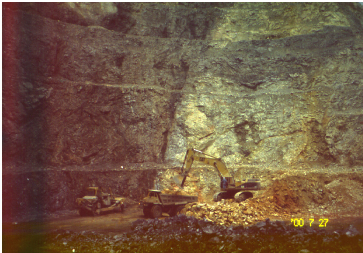
Figure 5. The Ursa fault sets gold-bearing graphitic limestone against light-coloured cherty dolomite near the bottom of the Ursa pit. Orientation of the Ursa fault changes upward from steep west dipping, as shown here, to steeply east near the surface.
