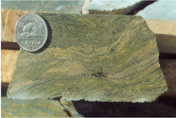
Photo 3. Close-up of auriferous pyrite mineralization from hole BC 2K-19, Bonanza Ledge zone.
