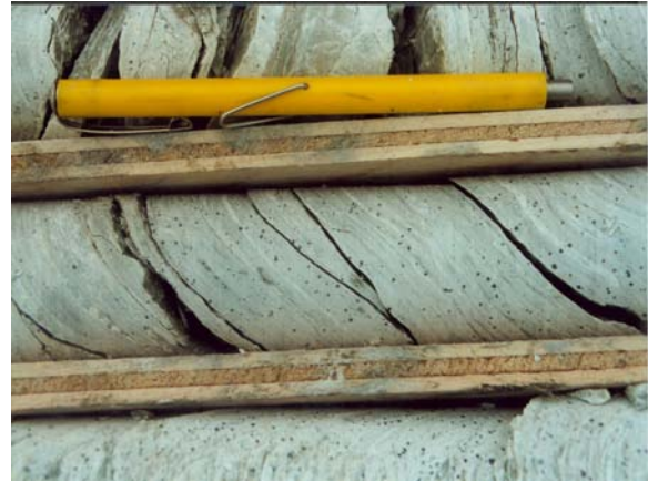
Photo 4. Close-up of hangingwall rocks with distinctive magnetite porphyroblasts (hole BC-2K-15), Bonanza Ledge zone.
