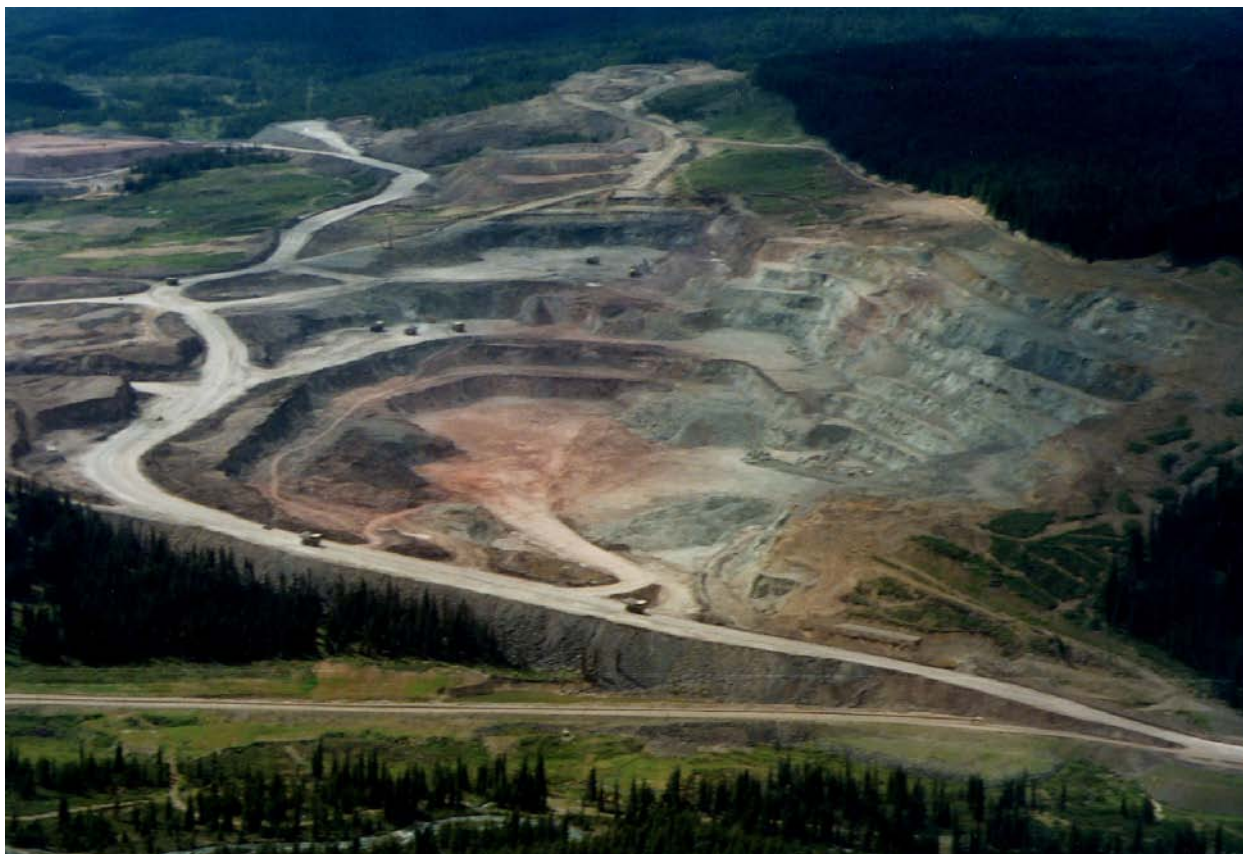
Photo 1. Looking westerly over the Kemess South orebody with waste rock dump in background. Two 240-tonne haul trucks in foreground provide scale (photograph taken by Ed Pittman, Inspector of Mines, Prince George).
