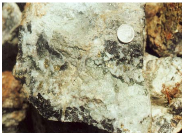
Photo 5. Sphalerite and chalcopyrite-bearing (dark clusters) epithermal quartz-carbonate vein, Stope Baby property.
