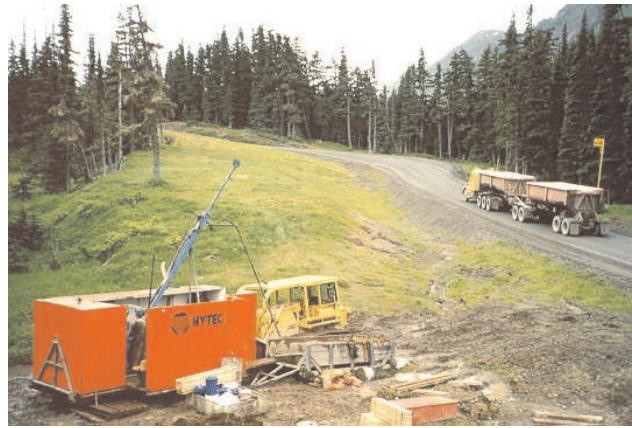
Photo 2. Exploration holes in the NEX zone are routinely drilled to 1500 metres. A truck departs the minesite carrying ore containing about $250 000 in gold and silver, destined for the DOWA or Noranda smelters.
