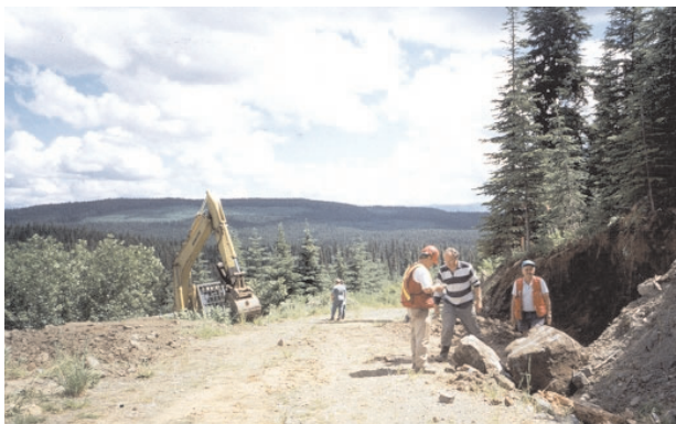
Photo 13. Geologists examine high-grade copper float in a trenched roadcut at the New Discovery “A” target on the Silver Lake property. Trenching below the road to the north (left) discovered vein-style quartz-carbonate-chalcopyrite-pyrite mineralization in bedrock.
