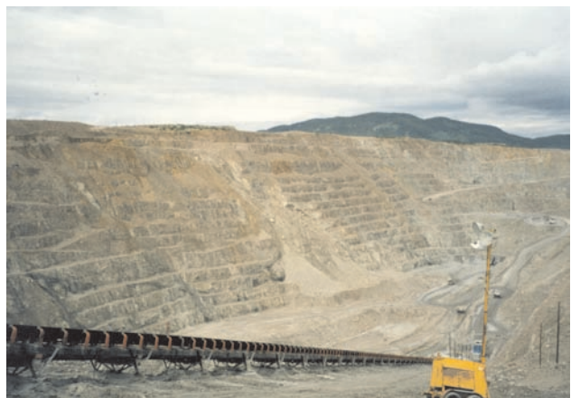
Photo 3. Endako open pit, showing the ore conveyor from the in-pit crusher and the area of instability on the south pit wall.
