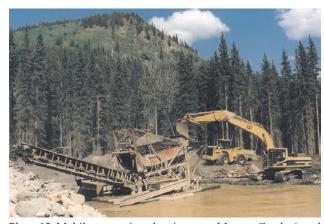
Photo 13. Mobile processing plant in use on Manson Creek, Angel Jade Mining.
