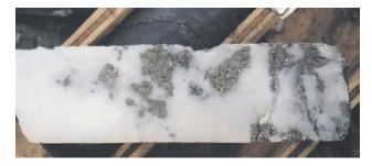
Photo 11. Quartz-pyrite vein mineralization from the Myrtle property.
