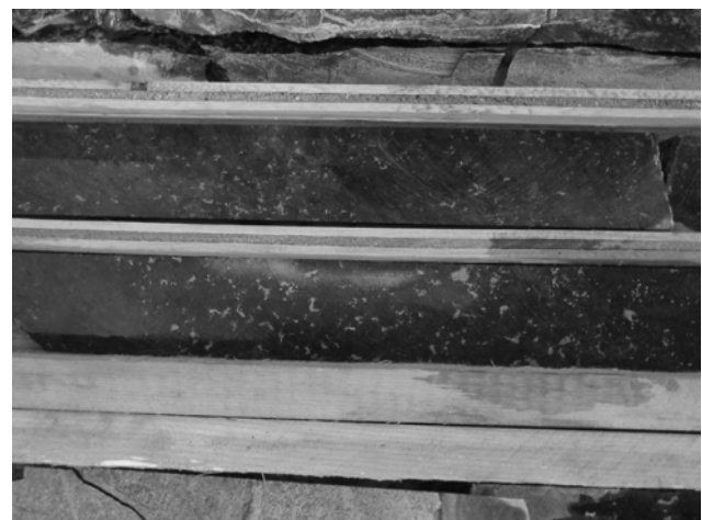
Photo 3. Turnagain property, drill hole 03-12; net-textured disseminated pyrrhotite and pentlandite in ultramafic rock.
