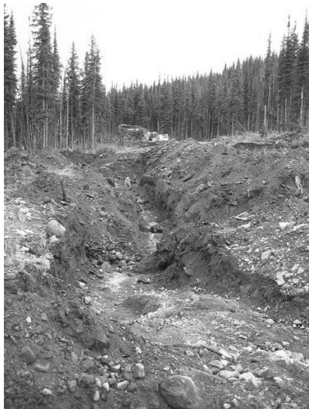
Photo 6. Trenching on the Eagle vein, Bonaparte gold property (courtesy North American Gem Inc.).
