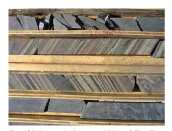
Figure 5-9: Laminated and massive sulphides in Sullivan Deeps SD#04-01 drill-core.
