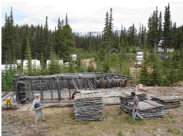
Figure 2.20. Lucky Ship molybdenum property, salvaging old drill core from collapsed racks.
