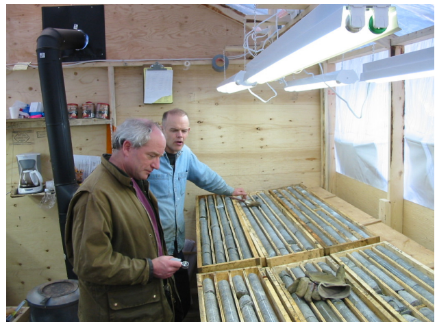
Figure 2.19. Geologists Hans Smit and Peter Daubney log core from the Seel porphyry copper property.
