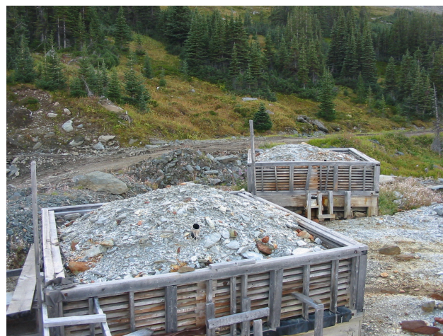
Figure 2.9. Kutcho Creek, cells to test for generation of acidic run-off water using rock from the adit, built in 1980s.
