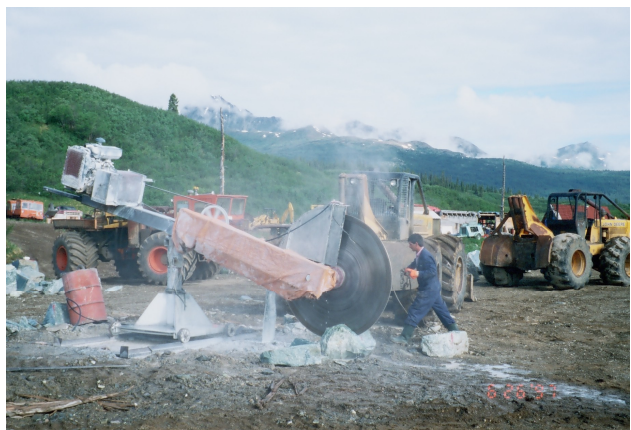
Figure 2.6. Near Provencher Lake, diamond-sawing jade blocks to assess quality.
