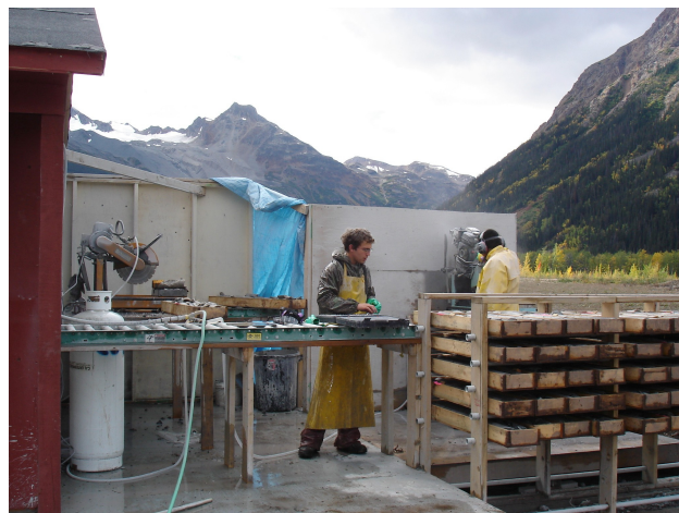
Figure 2.10. Schaft Creek, cutting P-size core to provide samples for assay and metallurgical study.
