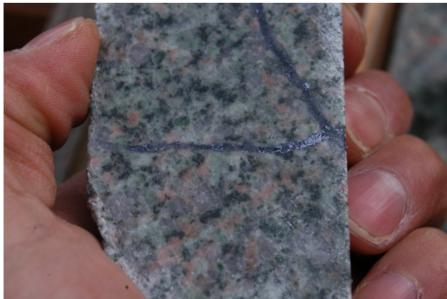
Figure 3.11. Fracture-controlled molybdenite in coarse-grained quartz monzonite, Nithi Mountain property.
