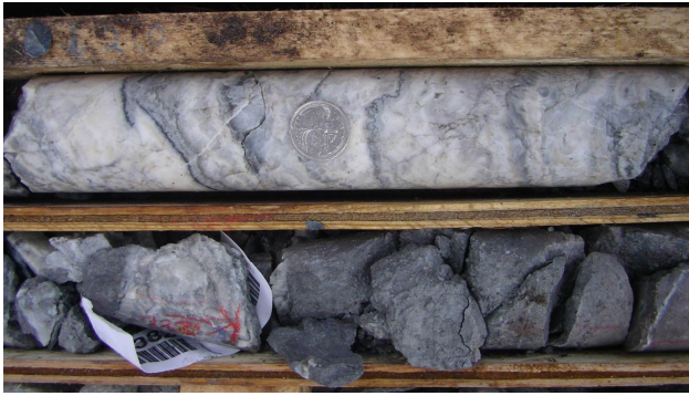
Figure 4.13. Banded epithermal quartz, Hole SC-007, Skoonka Creek property (section runs 47.8 g/t gold over 1.57 metres).
