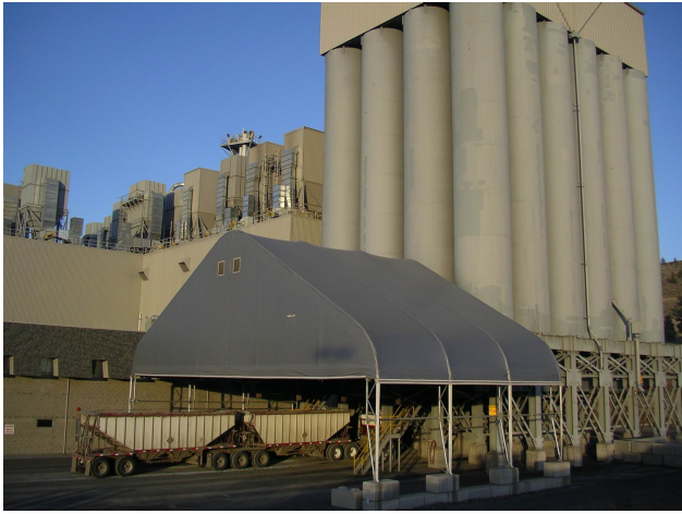
Figure 4.9. Truck arriving to pick up roofing granules at Ashcroft plant of IG Machine and Fiber Ltd.
