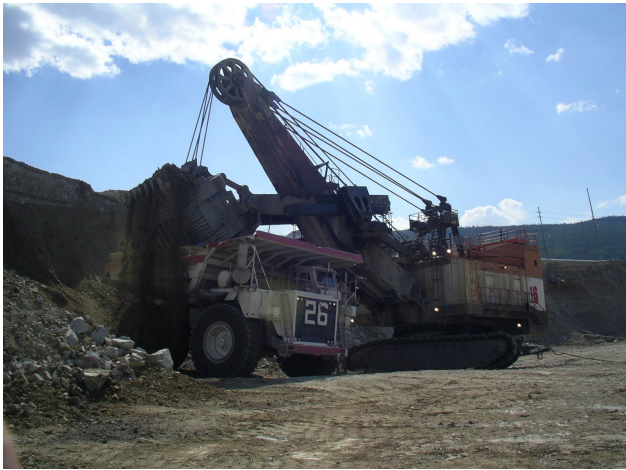
Figure 4.5. Stripping overburden at Valley pit, Highland Valley Copper.
