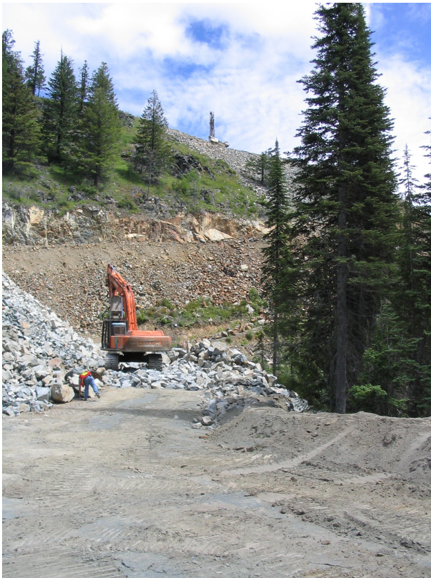
Figure 5.6. The Winner diorite quarry near Grand Forks, which provides feed for the Roxul (West) Inc rock wool plant in Grand Forks. The drill in the background is preparing for a blast.
