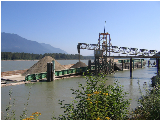
Figure 6.7. 1600 and 3100 tonne barges are loaded with aggregate at the Cox Station quarry of Mainland Sand & Gravel Ltd, located on the south side of the Fraser River at Sumas Mountain, central Fraser Valley.
