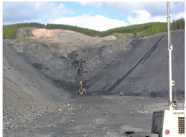
Figure 7.3. Coal extraction from both limbs of the syncline at the Dillon mine.
