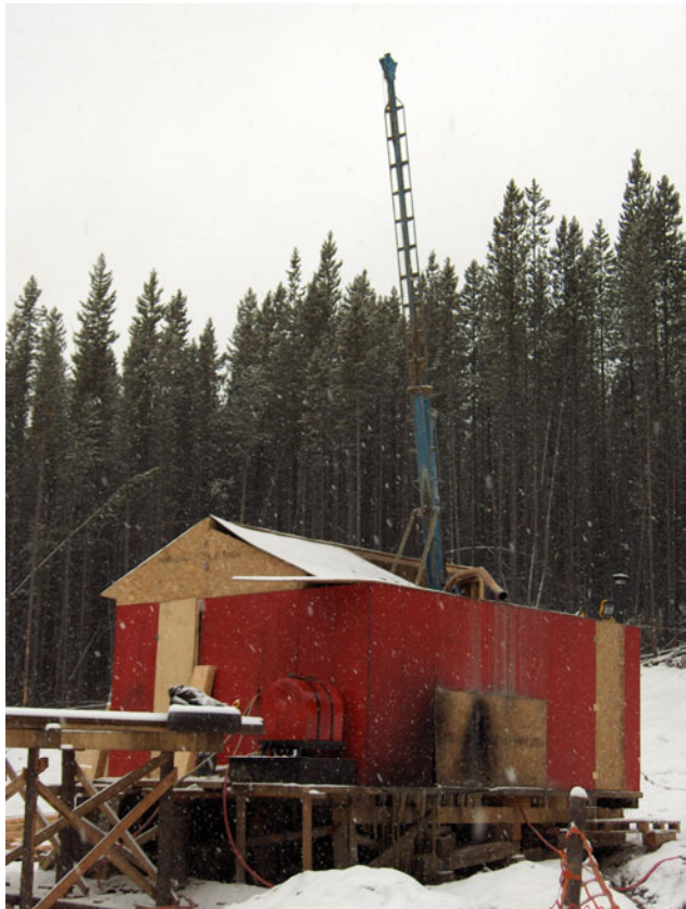
Photo 10. Sullivan Deeps property drillhole SD3 by Stikine Gold Corporation (photo by D. Grieve).
