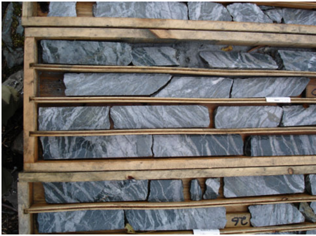
Figure 2.14. Intense quartz stockwork in drill core from the Mitchell zone, Kerr-Sulphurets property.
