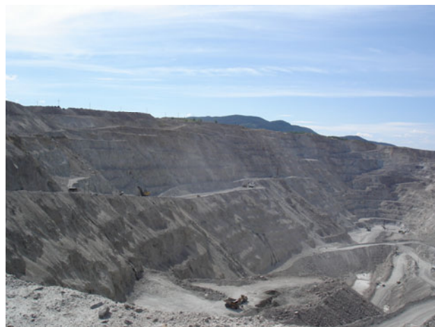
Figure 2.4. Benching the south wall of the Endako Pit.
