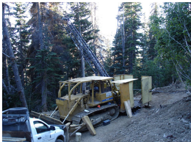
Figure 2.21. A diamond drill mounted on dozer at Lucky Ship.
