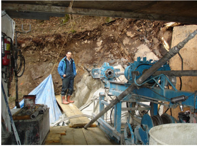
Figure 2.9. Jim Hutter at the collar of a flat drillhole - the pilot for a proposed lower adit for the Davidson deposit.
