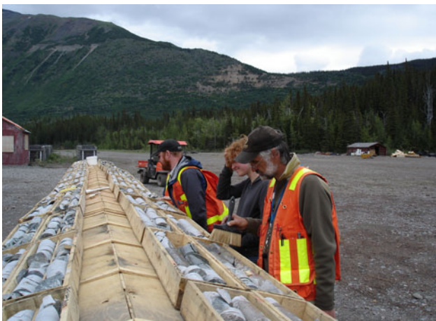
Figure 2.7. Logging P-size drill core with Schaft Creek copper deposit in the background.
