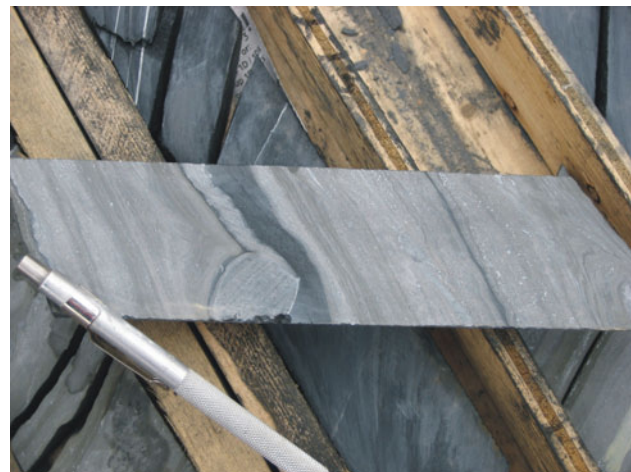
Figure 4.8. Laminated zinc-lead-silver sedex mineralization, Akie deposit.
