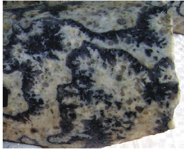
Figure 5.12. Unidirectional Solidification Texture quartz or "brain rock" from the Crazy Fox porphyry molybdenum-tungsten project (courtesy of Newmac Resources Inc).
