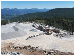
Figure 7.7. The Winner gabbro quarry near Grand Forks, which provides feed for the Roxul (West) Inc. rock wool plant in Grand Forks..
