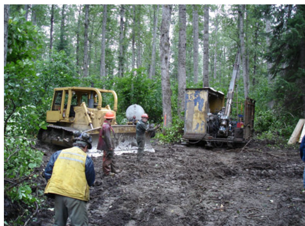
Figure 2.10. Richard Cote aligns a diamond drill at New Polaris.
