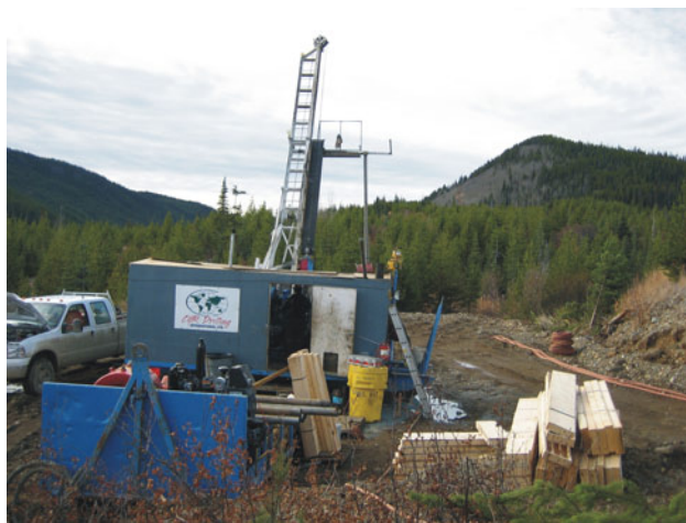
Figure 4.11. Large diameter core drilling of the MBX deposit, Mt. Milligan property.
