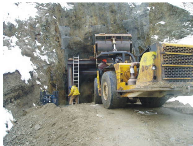
Figure 4.14. Development of the North zone portal, QR gold mine (photograph courtesy of Jim Miller-Tait).
