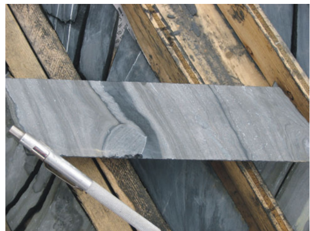
Figure 4.8. Laminated zinc-lead-silver sedex mineralization, Akie deposit.
