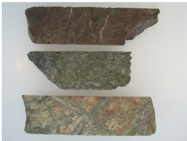
Photo 8. Hypogene copper-gold mineralization in core, drillhole K-06-09, Kwanika project. Top: Hematitic breccia with native copper fracture infillings. Middle: Quartz-sulphide (cpy-py)-tourmaline breccia. Bottom: Quartz-sulphide (cpy-py) stockwork in highly altered monzonite (photo courtesy of Serengeti Resources).
