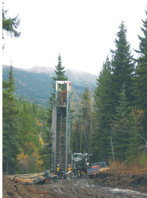
Figure 3.7. Air-rotary drilling to delineate coal resources, Horizon project.
