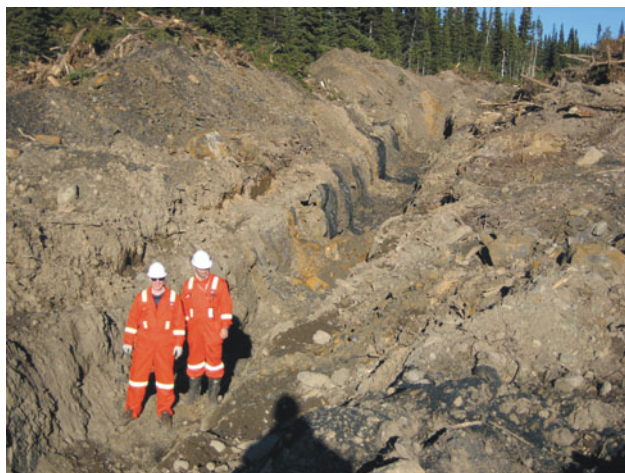
Figure 3.6. Trench exposing coal seams, Goodrich-Central South project.
