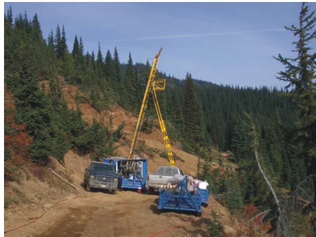
Figure 6.7. A diamond drill rig at Giant Copper (Photo by S. Robertson).
