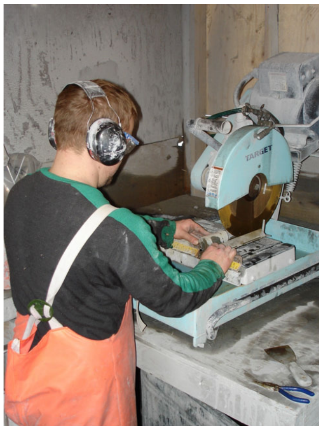
Figure 2.22. Cutting drill core with a diamond saw at the Seel property.
