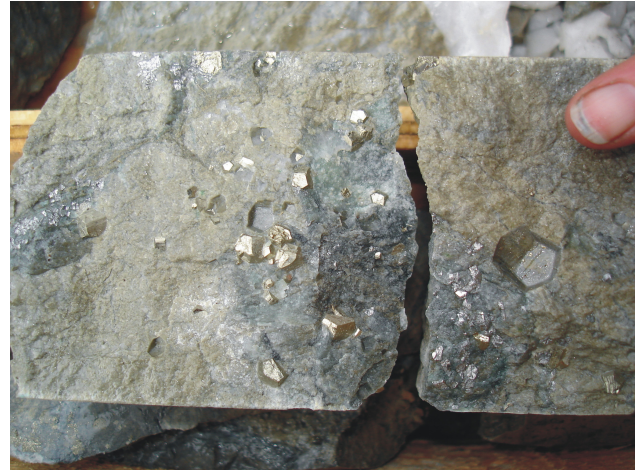
Figure 1.38. Pyritohedrons of pyrite in carbonate-altered basalt, Taurus project.
