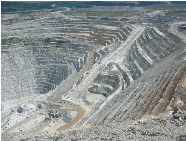
Figure 4.4. The Valley Pit at Highland Valley Copper showing trace of moved in pit conveyor and east wall overburden stripping.
