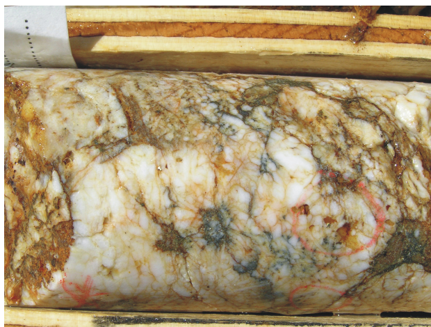
Figure 4.11. High-grade gold mineralization within quartz veins at the Elizabeth property of J-Pacific Gold Inc (Photo courtesy of J-Pacific Gold Inc).
