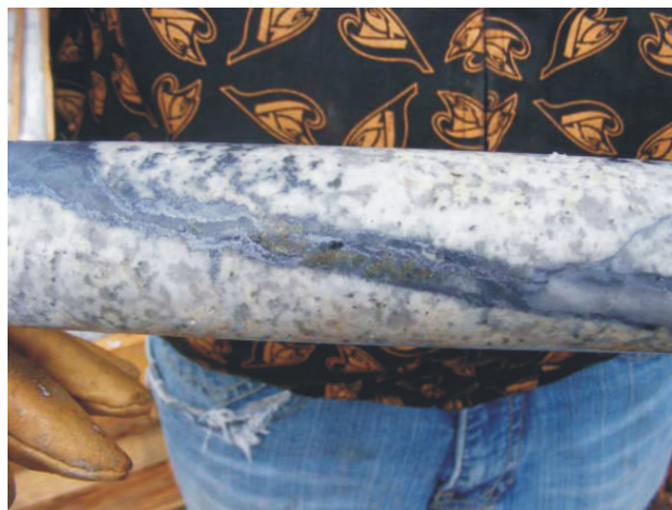
Figure 4.7. Strong molybdenite mineralization as both fracture filling and disseminations below the offsetting thrust fault at the Crazy Fox (Photo courtesy of Newmac Resources Inc).
