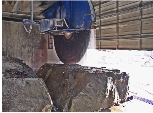
Figure 5.9. A piece of Haddington Island under the 11 foot saw at Bedrock Granite Sales Ltd.
