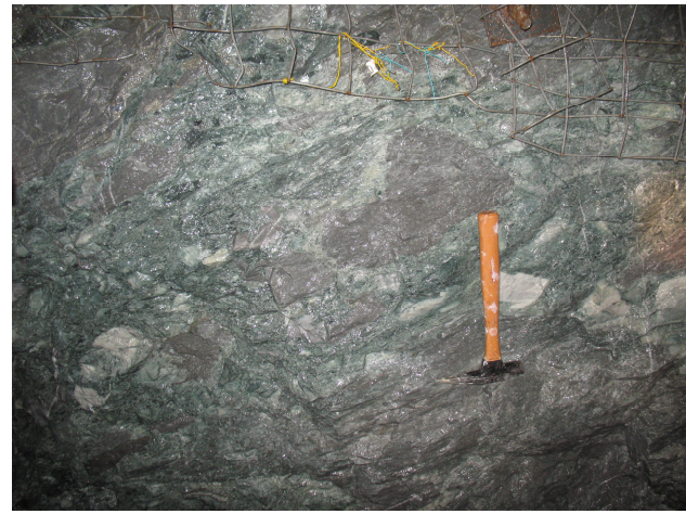
Figure 5.4. Ore clast breccia, H-W mine, Myra Falls.
