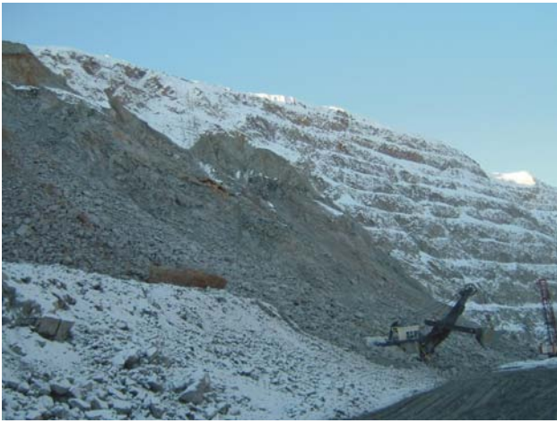
Figure 1.3. Mining equipment was trapped temporarily but not damaged by the Nov. 12 slide in the Endako Pit.
