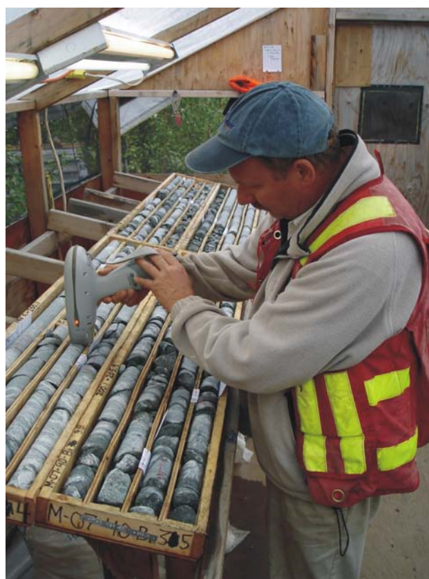
Figure 1.20. Portable XRF analyzer gives immediate indication of copper, and by inference the gold grade of Mitchell zone drill core.
