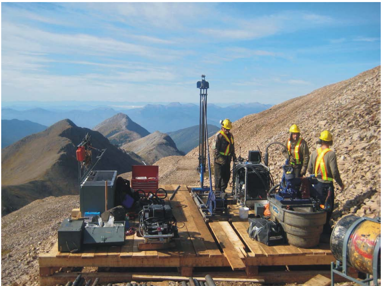
Figure 3.13. Heli-supported drilling at the Aley project.
