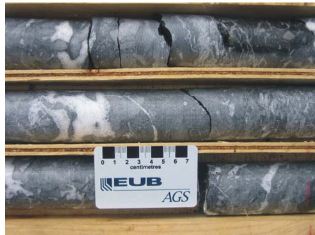
Figure 3.17. Stromatoperoid boundstone in core from the Pat (Giscome) project (courtesy Graymont).
