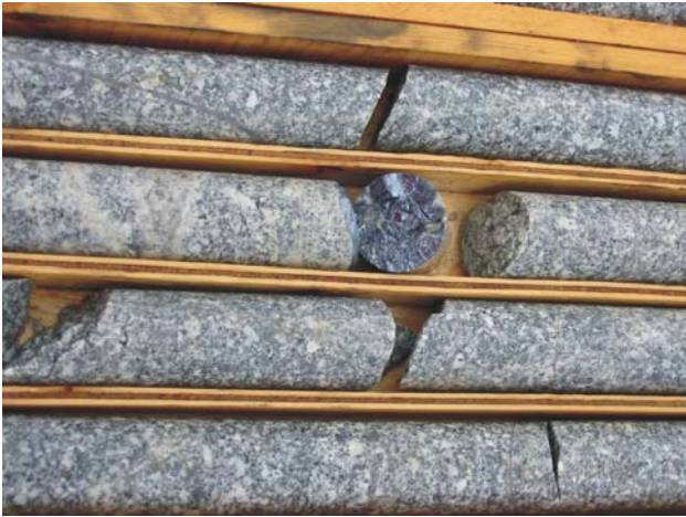
Fig 1.11. Molybdenite vein in coarse-grained granite, Ruby Creek deposit.
