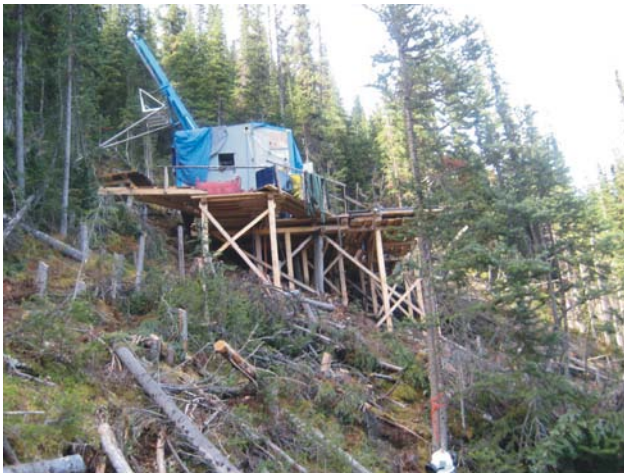
Figure 3.12. Drilling platform at the Akie project.
