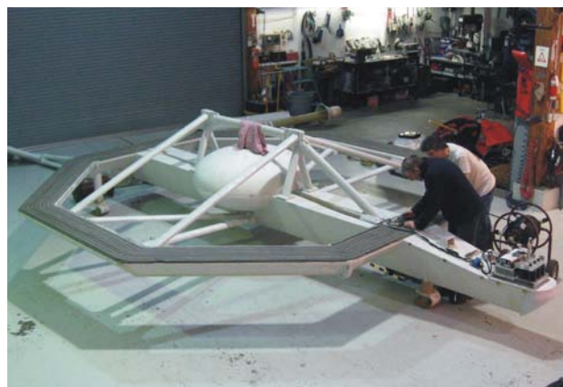
Figure 4.9. Technicians at Aeroquest International Ltd prepare the AeroTEM II for helicopter mounting and airborne EM and Magnetic surveys of the Tasco, Yalakom and Piebiter properties in the southern Chilcotin and Bralorne area (Photo courtesy of John Chapman).
