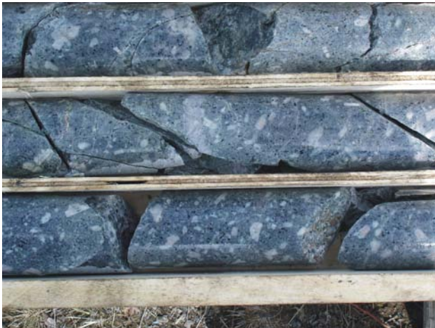
Figure 1.30. Swan, a porphyritic phase of the Glundebery batholith in drill core, with prominent potassium feldspar.
