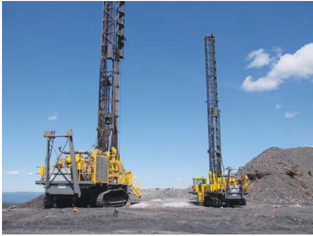
Figure 2.5. New “Pit Viper” blast hole drills at the Trend Mine.
