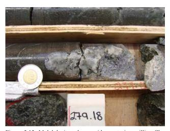
Figure 3.13. Molybdenite selvage with quartz in argillite, Chu project.
