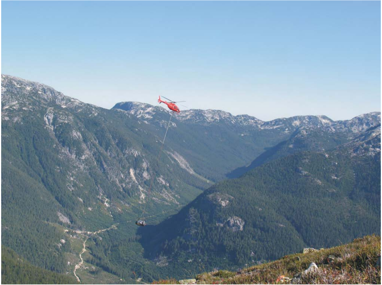
Figure 5.13. Slings with a long line at the Crack molybdenum project. Despite an extensive road network, the rugged terrain (and road deactivation) necessitated helicopter support for several projects on the east side of Harrison Lake.
