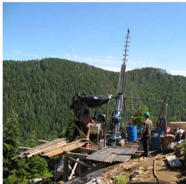
Figure 5.9. A helicopter-portable drill rig on the Cliff zone at Catface Copper.
