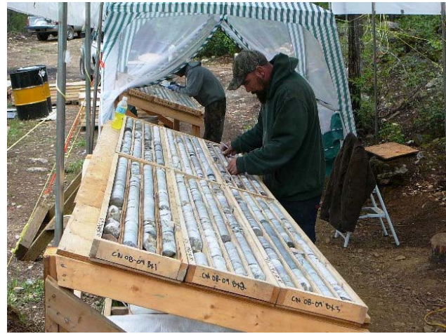
Figure 4.14. Core logging at the CK project of CMC Metals Ltd located between Clearwater and Blue River along the Raft River.
