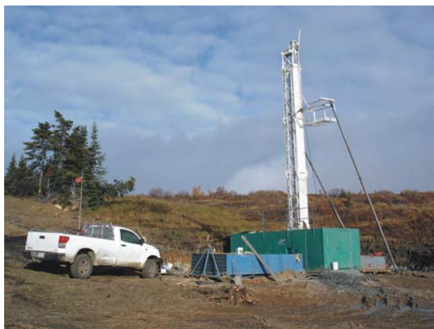
Figure 1.19. Red Chris, Boyles 56-model drill, capable of drilling to 1500 m.
