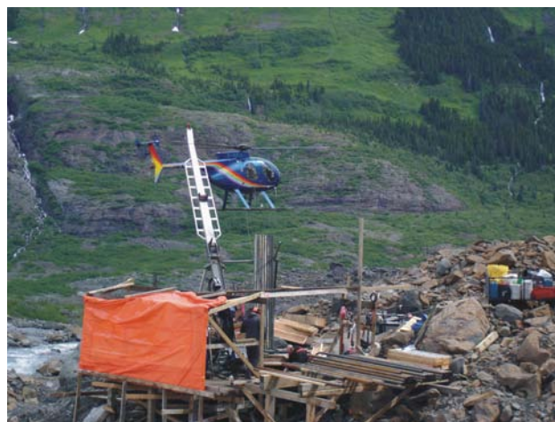
Figure 1.52. Homestake Ridge, helicopter-supported drilling near the toe of the Homestake glacier.
