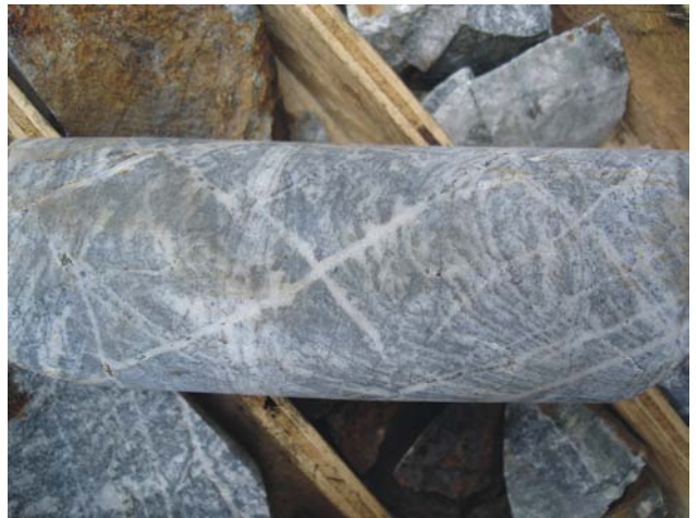
Figure 1.21. Bronson Slope, quartz-magnetite vein stockwork and replacement.
