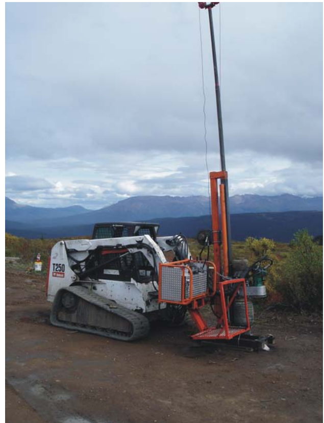
Figure 1.10. Red Chris, innovative mobile drill designed for short core holes to explore the till-covered Todagin plateau.
