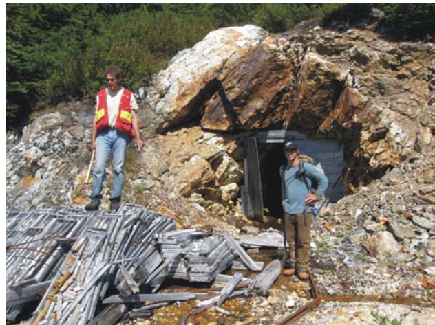
Figure 1.26. Deer Horn, Harry Huffels and Cody Philpott at the adit and collapsed 1989-1990 drill core; the moderately dipping quartz-gold vein is visible above the portal.
