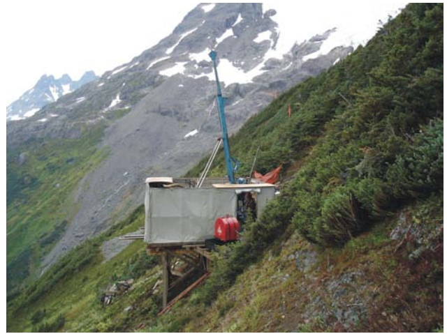
Figure 1.20. Trek, drilling a copper-gold breccia from a steep slope set-up.
