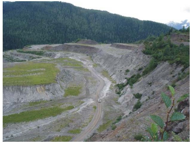
Figure 1.15. Kitsault open pit, molybdenum ore forms an annular zone between the barren core of the stock (left) and hornfelsed sedimentary rocks (right).
