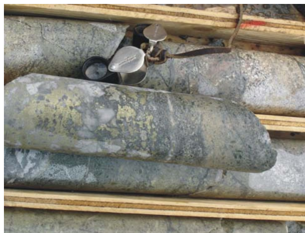
Figure 1.22. Zymo, chalcopyrite and quartz in an altered, even-grained diorite.
