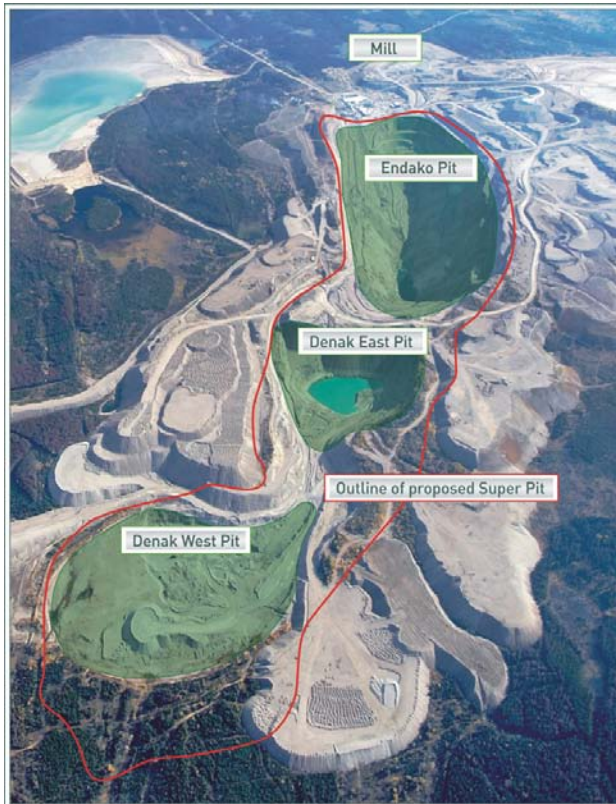
Figure 1.6. Endako molybdenum mine, aerial view of super-pit that will incorporate Endako, Denak East and Denak West, north is to the left.
