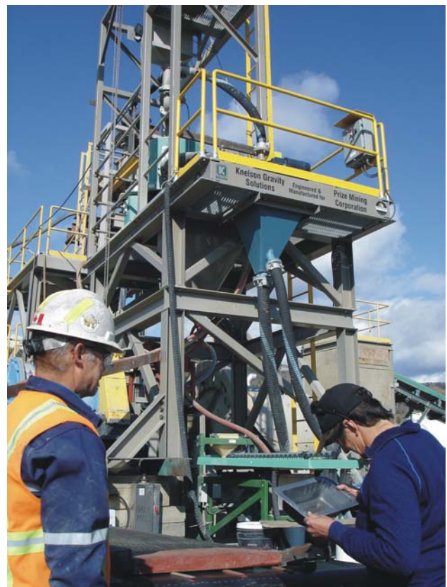
Figure 1.7. Yellowjacket gravity mill treating gold ore.
