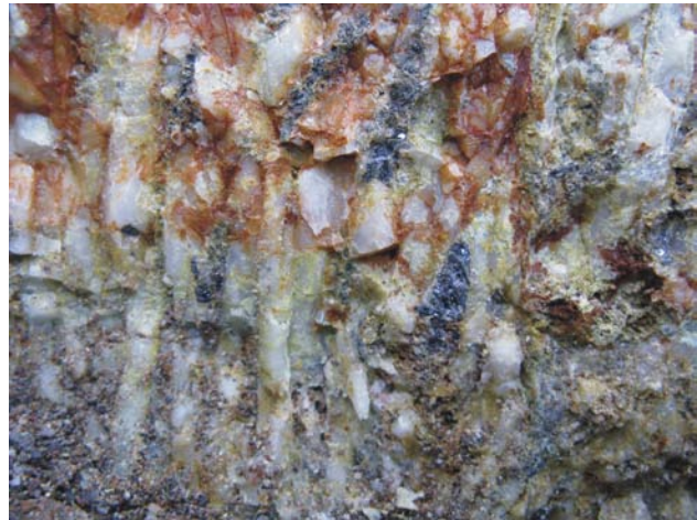
Figure 4.18a. A close up of a gold-silver-bearing quartz sulphide vein at the Watson Bar property. Photos for Figures 4.18 a, b and c courtesy of Durfeld Geological Management Ltd.
