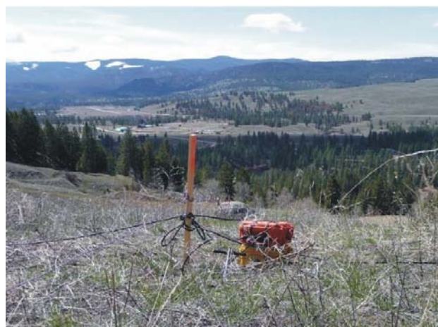
Figure 4.15. A Quantec Titan-25 deep penetrating IP survey set up at the Miner Mountain project just north of Princeton (photo courtesy of Sego Resources Inc).
