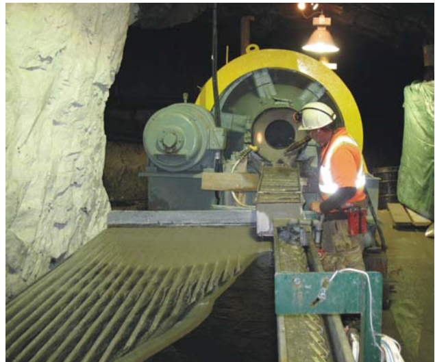
Figure 5.15. The ball mill and gravity table used to process a bulk sample at the Mineral Creek project.
