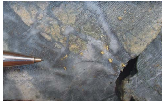
Figure 5.16. Visible gold in drill core from the Ember vein, Mineral Creek project.
