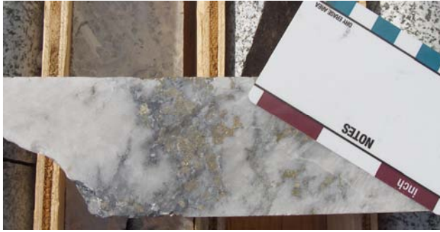
Figure 6.13. Sulphide minerals in quartz vein material in drill core at the Kenville Gold Mine property. Eagle Creek intrusive material is visible adjacent to the scale card.
