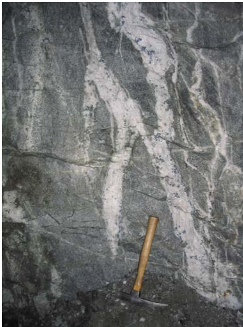
Figure 6.6. Molybdenite-bearing quartz vein stockworks underground at the Roca Mines Inc MAX molybdenum mine.
