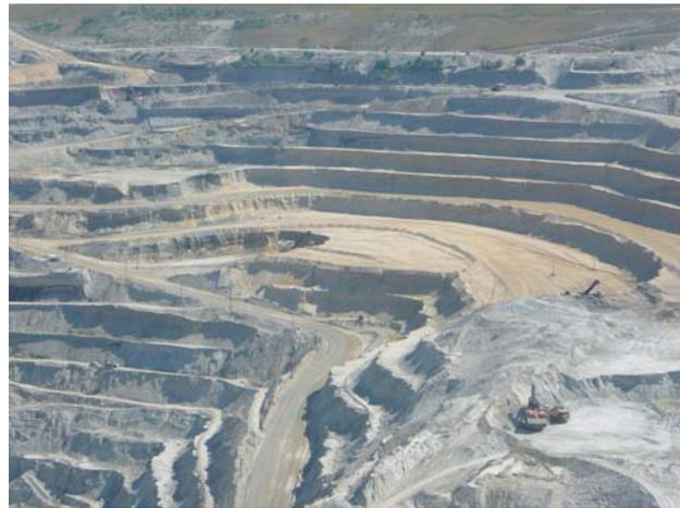
Figure 4.5. Overburden stripping at the east wall expansion of the Valley pit at the Highland Valley Copper mine near Logan Lake.
