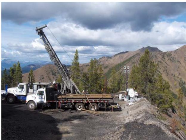
Figure 6.9. View looking north of rotary drilling at the north end of Teck Coal Limited's Mount Michael property.
