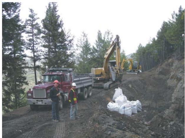
Figure 4.18c. At the Watson Bar property. Loading the bulk sample into a haul truck in preparation for direct shipping to the custom mill.
