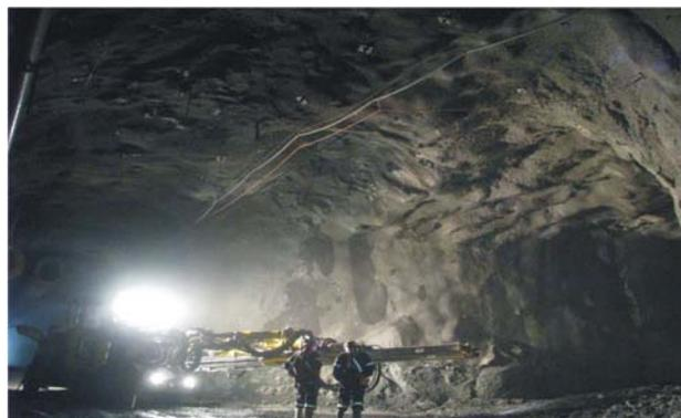
Figure 4.9. A Jumbo at the New Afton mine development site which now includes over 5 km of underground development and a 4.5 km conveyor decline that is nearing completion (photo courtesy of New Gold Inc).
