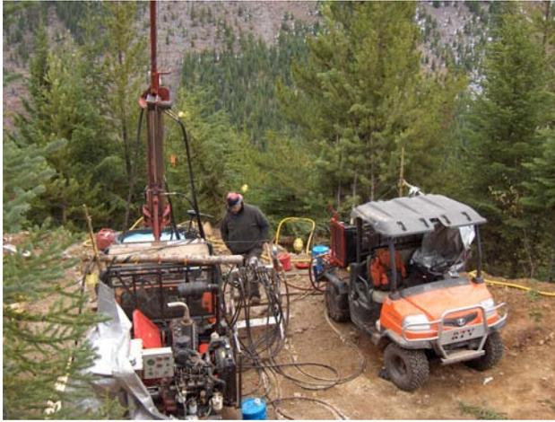
Figure 6.20. Diamond drilling on Spectrum Mining Corporation's Rock Canyon Creek project.
