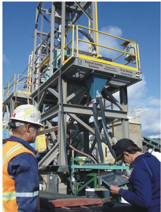
Figure 1.7. Yellowjacket gravity mill treating gold ore.
