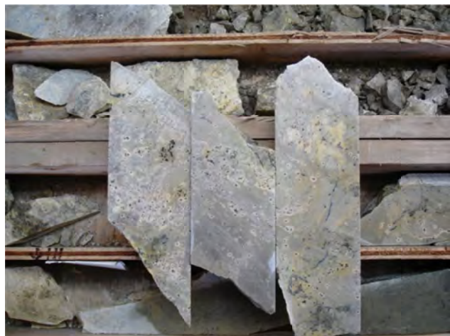
Figure 19. Blackwater-Davidson Hole 63, black sulphide 'specks' and 'dendrites' surrounded by silica coronas; part of 312 m interval that grades 0.76 g/t Au.
