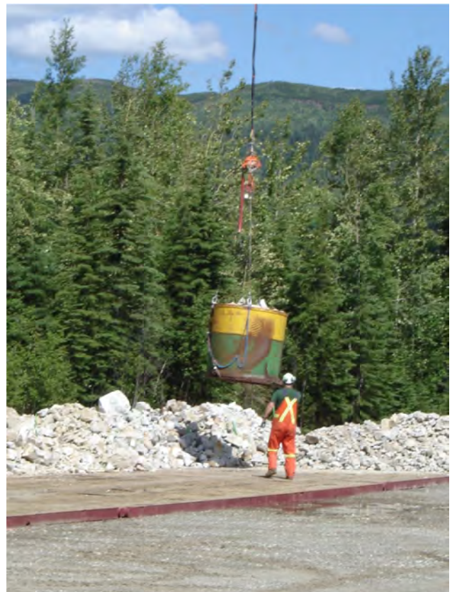
Figure 34. Staging point for Nonda bulk sample, storage on a prepared platform to avoid contamination.
