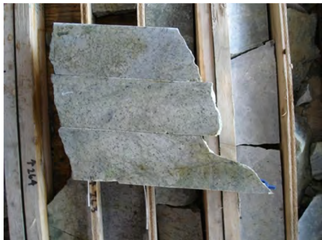
Figure 20. Blackwater-Davidson Hole 68, black sulphide 'specks' and 'dendrites' with faint breccia texture in rhyolite; part of 227 m interval that grades 1.51 g/t Au.
