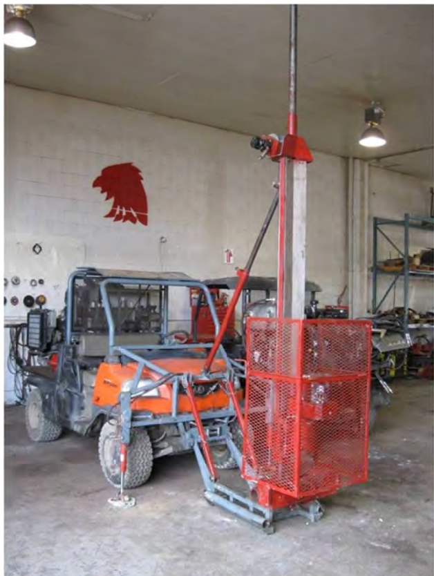
Figure 11. Kubota-mounted diamond drill used in the Prince George Porphyry project.
