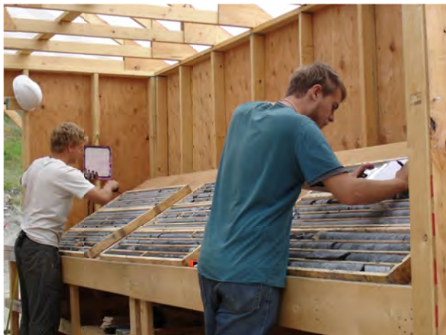
Figure 15. Darcy Vis and Ian Carr prepare geotechnical and geological core logs at Decar.
