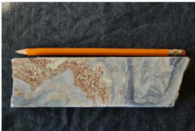
Figure 32. Carbo hole 6 at 149.7 m, cumulate layer of bastnaesite, a REE carbonate mineral, image courtesy of Allison Brand.
