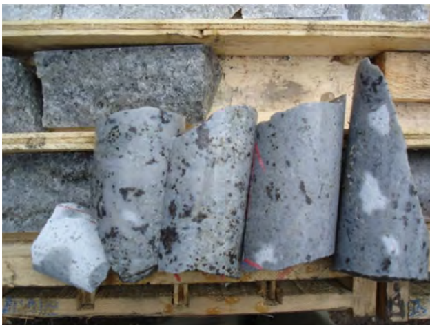
Figure 25. Capoose Hole 127, specimens from an interval rich in garnet, note anhedral shape.
