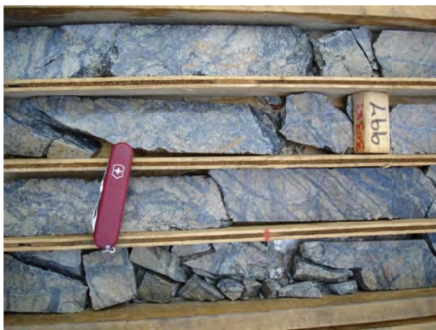
Figure 10. Kwanika Central zone, supergene chalcocite in quartz stockwork with overprint of albite-Fe-carbonate-hematite alteration, from drillhole 62.
