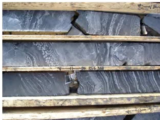
Figure 28. Akie, delicate laminae and pearl-like beads of barite in the hangingwall shale of the Cardiac Creek SEDEX deposit.
