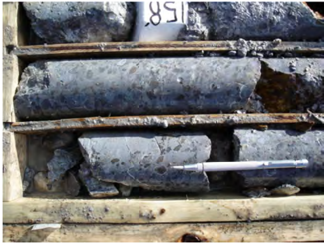
Figure 21. Blackwater-Davidson Hole 68, rhyolite breccia with grey silica clasts, brown sphalerite clasts and pale kaolin clasts; kaolin rims on many clasts; part of a 67 m interval that grades 0.59 g/t Au.
