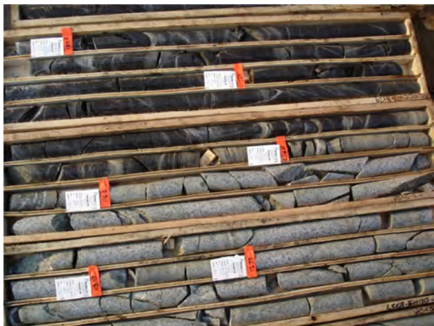
Figure 85. Sidina gold project; quartz-sulphide vein at the contact between biotite hornfels and granodiorite.
