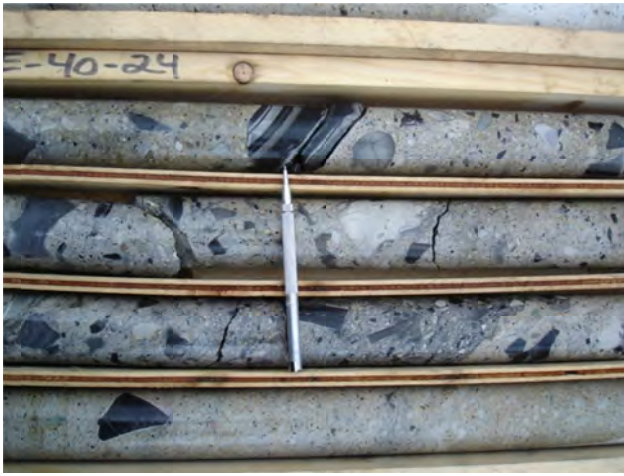
Figure 88. Coles Creek project; rhyolite epiclastic breccias with locally abundant mudstone cobbles in the Kasalka Group.
