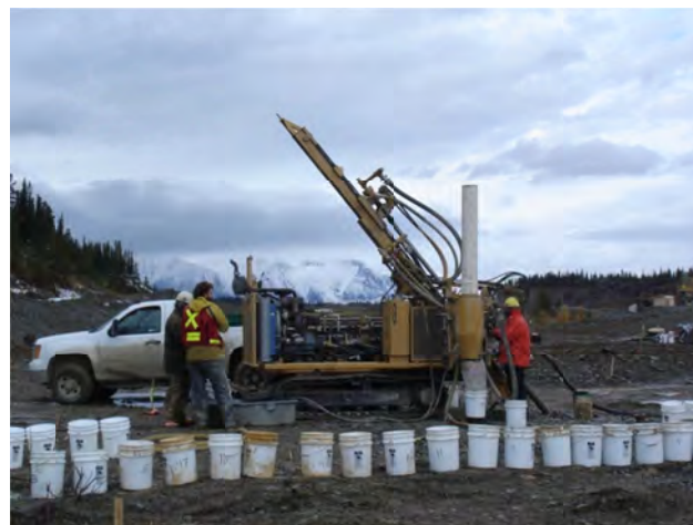
Figure 13. Yellowjacket gold project; reverse circulation drill on an angle hole in the historic placer channel of Pine Creek.
