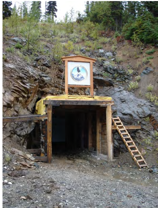
Figure 11. Dome gold mine in September 2011, portal of the refurbished 1290-level, to be the main production level.
