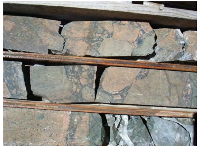
Figure 23. Schaft Creek copper project; West Breccia zone in hole CF-326, angular hematite-altered fragments.
