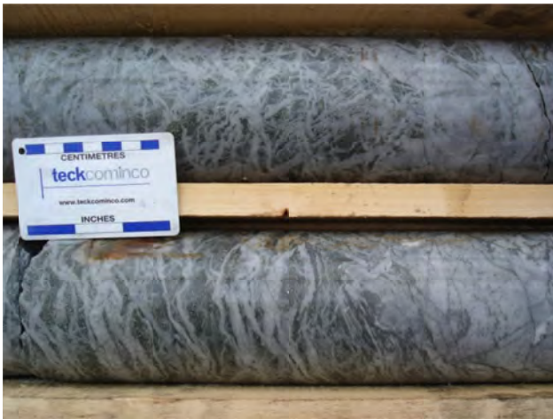
Figure 42. Snowfield project; intense and deformed quartz stockwork of Main (North) Snowfield gold-copper zone, PQ core from a metallurgical hole.
