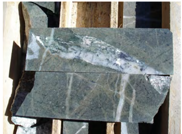
Figure 25. Schaft Creek copper project; Liard zone, altered feldspar in an intrusive rock with quartz-bornite vein, hole CF-347.
