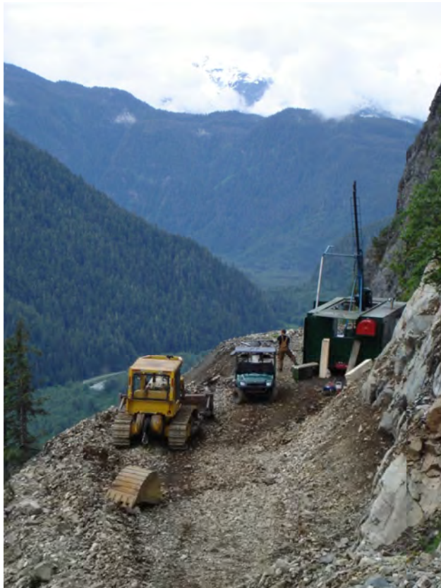
Figure 79. Red Cliff gold project above American Creek north of Stewart; a steep slope drill set up.
