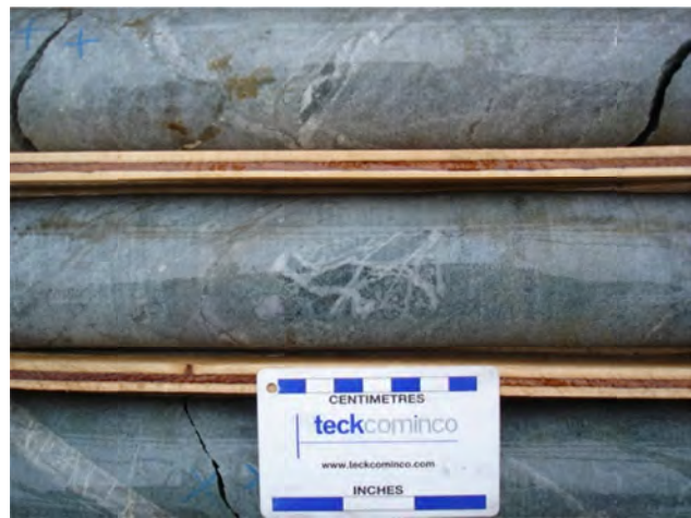
Figure 44. Snowfield project; fragment of deformed stockwork typical of the Main zone in the non-strained Upper zone. Implies a post-deformation origin to the Upper zone.
