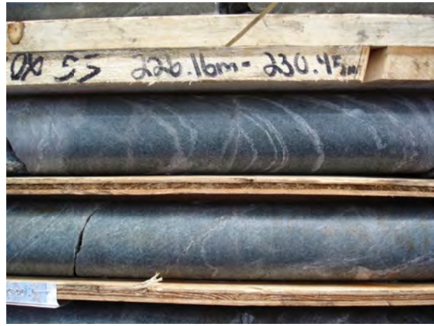
Figure 43. Snowfield project; MZ-117 at 228 m, quartz-sulphide veins in chlorite alteration, interval grades 0.44 g/t Au, 0.13% Cu, at southeast margin of the Main zone.
