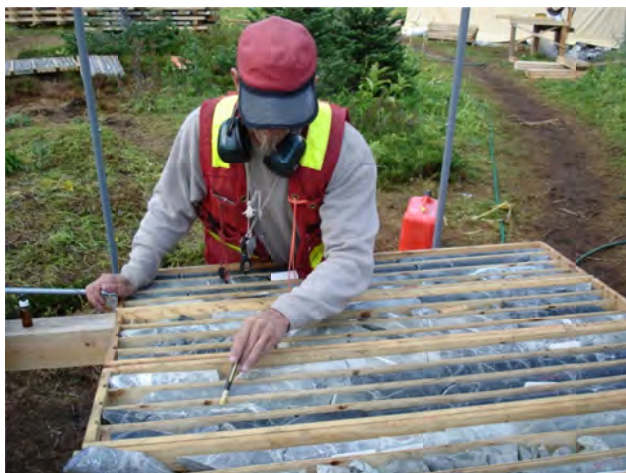
Figure 52. High Gold project; geologist Dan Meldrum logging drill core.
