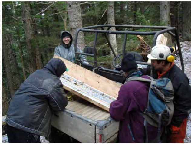
Figure 84. American Boy project; geologist Andris Kikauka (purple fleece) inspects drill core to advise Dwight Harvey (driller, white hat) if the hole is terminated. Crew members Otto Paeseler and Neil Johnson look on.
