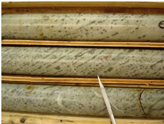
Figure 37. Brucejack project; West zone SU-100 at 535 m, quartz-sericite-pyrite alteration, with relict sedimentary bedding?.
