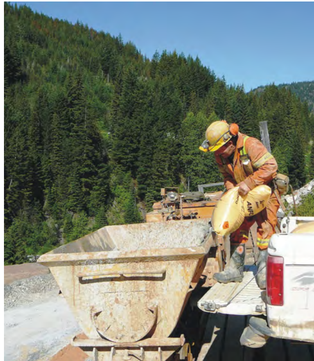
Figure 27. Loading explosives into an ore cart at the Bralorne mine.
